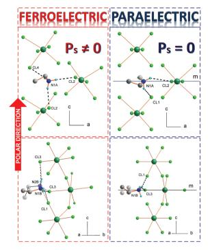
Fig. 3 The details of the cation arrangements in both phases. In paraelectric Phase I, both cations A and B are disordered over the ..m mirror plane with the 0.5/0.5 occupancy ratio; in ferroelectric Phase II, the A moiety is ordered, whereas the B takes two independent spatial orientations with the 0.6/0.4 occupancy ratio at 100 K. Dashed lines stand for hydrogen bonds.
