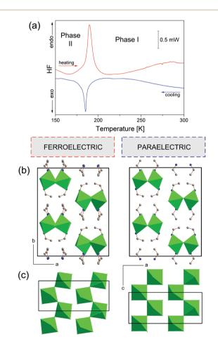
**Fig. 1** (a) DSC data confirming the transition sequence seen in **ECB** (rate: 10 K min<sup>-1</sup>, sample mass: 12.86 mg); (b) the structure overview of the paraelectric Phase I (right) and ferroelectric Phase II (left); (c)  $[\operatorname{BiCl}_5]^{2-}_{\infty}$  chains propagate along the c-direction and distinctly deform after the PT.
