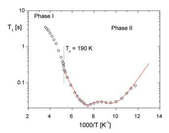
Fig. 4 Temperature dependence of the spin-lattice relaxation time  $(T_1)$ of <sup>1</sup>H NMR; the solid line represents the best fit calculated using egn (1) in ESI, Part 5.†
