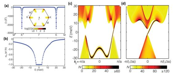
Fig. 5 (a) The distribution of the Berry curvature in momentum space for NiCl<sub>3</sub>. (b) Anomalous Hall conductivity when the Fermi level is shifted from its original Fermi level. Calculated local density of states of edge states for (c) zigzag and (d) armchair insulators. The edge states are calculated on the edge of a semi-infinite plane. The warmer colors (darker) represent higher local density of states at the edge.
