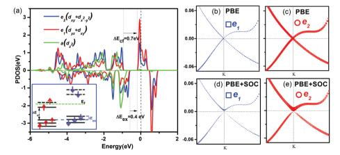
Fig. 6 (a) The PDOS of d states for Ni atoms is shown. The schematic figure (inset in part a) is the crystal field splitting and exchange splitting for Ni ions. (b) The evolution of orbital-resolved band structures ( $e_1$  and  $e_2$  states) of a NiCl<sub>3</sub> monolayer without and with SOC. The Fermi level is set to zero.
