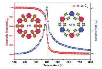
Fig. 3 Variations of the average magnetic moment (red) and specific heat (blue) calculated for a NiCl<sub>3</sub> monolayer with respect to the temperature. Spin-polarized charge densities with spin directions for NiCl<sub>3</sub> are shown in insets (blue dotted areas depicts the spin up); iso-surface value of +0.005 e  $Å^{-3}$  is shown.
