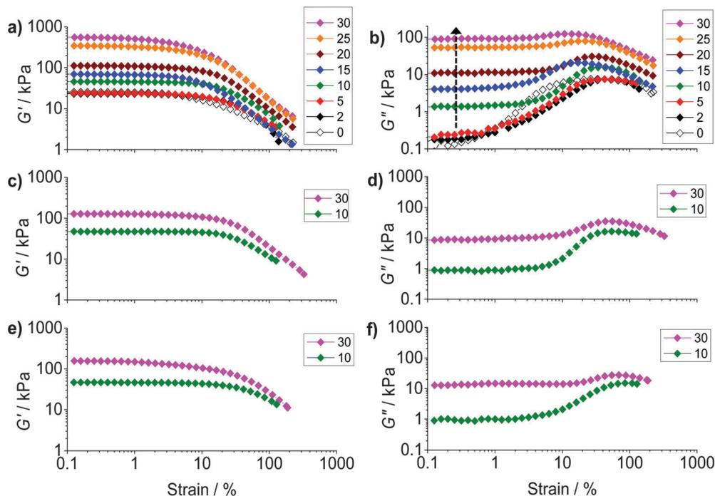
Fig. 5 Strain-sweep rheology study. Data for  $G'$  (left column) and  $G''$  (right column) are shown as a function of strain for PAAm/HP<sub>XL(y)</sub> (a and b), PAAm/HP<sub>VF(y)</sub> (c and d) and PAAm/HP<sub>(y)</sub> (e and f). The values for  $y$  are shown in the legends. The arrow in (b) highlights the increase for  $G''$  at low strain with increasing  $y$ .
