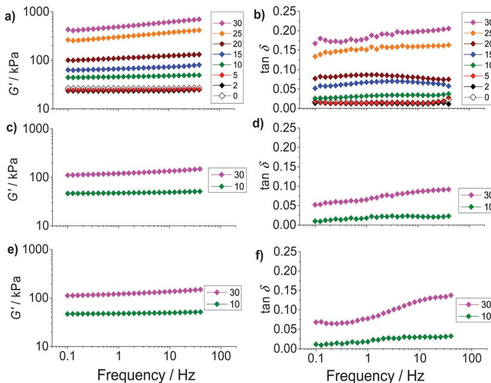
Fig. 3 Frequency-sweep rheology study. The variations of  $G'$  (storage modulus) and  $\tan \delta (=G''/G')$ , where  $G''$  is the loss modulus) with frequency are shown in the left and right columns, respectively, for PAAM/HP<sub>XL(y)</sub> (a and b), PAAM/HP<sub>VF(y)</sub> (c and d) and PAAM/HP<sub>(y)</sub> (e and f). The legends show the values for  $y$  (%).
