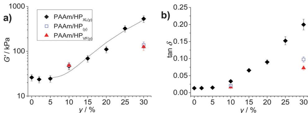
Fig. 4 Effects of hollow particle concentration on gel mechanical properties. The variations of (a)  $G'$  and (b)  $\tan \delta$  with particle concentration ( $y$ ) are shown for the three composite gels. The data have been taken from Fig. 3. The legend applies to both graphs. The curve in (a) is the fit from eqn (1). The value for  $A$  was 0.10.
