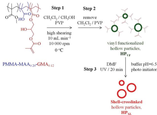
**Scheme 1** Hollow particle preparation. Depiction of preparation of hollow particles containing unreacted vinyl groups (HP<sub>VF</sub>) and shell-crosslinked hollow particles (HP<sub>XL</sub>). Hollow particles that did not contain pendant vinyl groups (HP) were also prepared. In that case PMMA-MAA<sub>0.35</sub> was used as well as steps 1 and 2.
