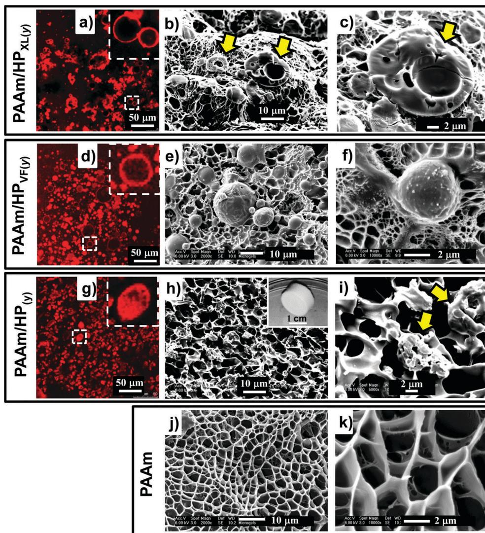
**Fig. 2** Composite gel morphologies. The identities of the gels are shown on the left hand side of each row. CLSM images are shown in (a), (d) and (g). The remaining images are from SEM of freeze-dried samples. The inset of (h) shows a free-standing gel. The values of  $y$  for all of the composite gels were 10 with the exception of (d) and (g), where the  $y$  values were 20. The arrows in (b), (c) and (i) identify hollow particles.
