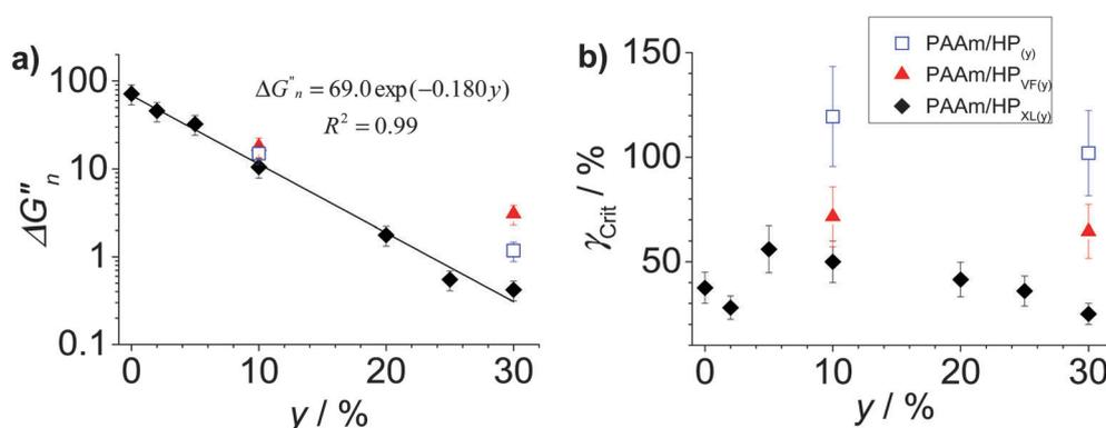
Fig. 6 Effects of particle concentration on gel dissipation and ductility. (a) Variation of  $\Delta G_n''$  ( $= (G_{\text{peak}}'' - G_o'')/G_o''$ ) where  $G_{\text{peak}}''$  and  $G_o''$  are maximum  $G''$  and strain-independent  $G''$  values, respectively) and (b) Variation of  $\gamma_{\text{crit}}$  with particle concentration ( $y$ ) for the composite gels. The data have been taken from Fig. 5.
