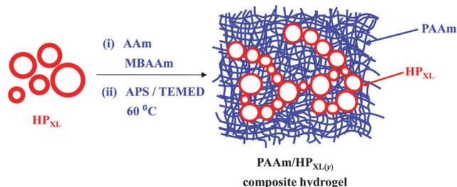
**Scheme 2** Composite gel preparation. Depiction of the procedure used for the preparation of PAAm/HP<sub>XL(y)</sub> composite gels. The same method was also used for the preparation of PAAm/HP<sub>VF(y)</sub> and PAAm/HP<sub>(y)</sub> gels.
