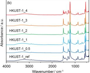
Fig. 4 FT-IR spectra of (a) the solvent insoluble Cu-based precursors (Cu-based precursors\_X) and (b) corresponding HKUST-1\_X with HKUST-1\_ref.
