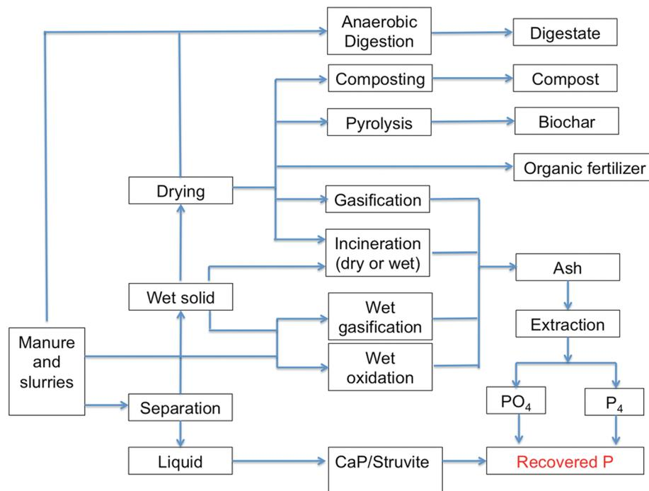
Fig. 4 Schematic overview of the main options to recover P from manures and biosolids. Adapted from Oenema et al.<sup>53</sup> and Schoumans et al.<sup>55</sup>
