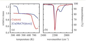
Thermogravimetric behaviour of Cu(tcm) [Cu(MeCN)(tcm)]. The mass loss observed near 400 K for the latter corresponds to volatilisation of one molar equivalent of MeCN. Both TGA curves have been normalised to the mass measured at 420 K (b). High-frequency region of the infrared absorption spectra of Cu(tcm) and [Cu(MeCN)(tcm)] showing the emergence of an additional band in the latter, attributed to the nitrile C-N stretch. Colour scheme as in (a).
