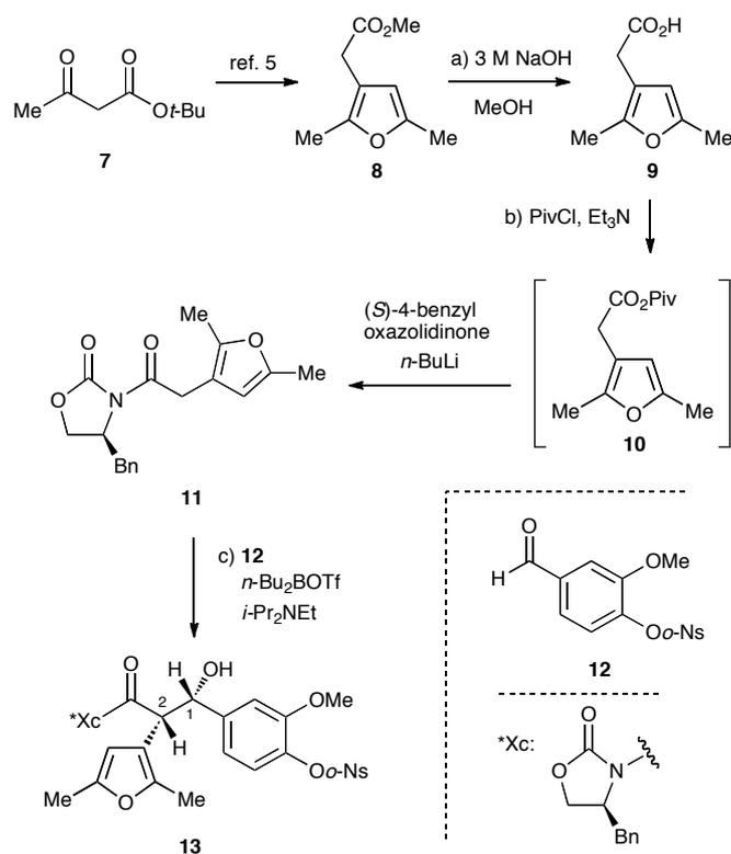
**Scheme 2.** Synthesis of key intermediate **13** via *syn*-selective Evans aldol reaction. Reagents and Conditions: a) 3 M NaOH aq., MeOH, rt, 2 h, quant.; b) PivCl, Et<sub>3</sub>N, THF, -78 °C to 0 °C, 1 h, then (S)-4-Bn-oxazolidinone, *n*-BuLi, THF, -78 °C to 0 °C, 1 h, 93%; c) *n*-Bu<sub>2</sub>BOTf, *i*-Pr<sub>2</sub>NEt, **12**, CH<sub>2</sub>Cl<sub>2</sub>, -78 °C, 2.5 h, 98%, d.r. >95:5. Piv: pivaloyl; Bn: benzyl; *n*-Bu<sub>2</sub>BOTf: di-*n*-butylboryl trifluoromethanesulfonate.
