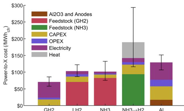
**Fig. 9** PtX cost distribution for all carriers at \$30/MWh<sub>e</sub> electricity cost. Error bars reflect the uncertainty from all PtX input parameters (see Table 3). The gaseous hydrogen (GH<sub>2</sub>) stack refers to the hydrogen production cost from the electrolyser then used as a feedstock for LH<sub>2</sub> and NH<sub>3</sub>, which totals \$70.5/MWh<sub>ch</sub> or \$2.35/kgH<sub>2</sub>.
