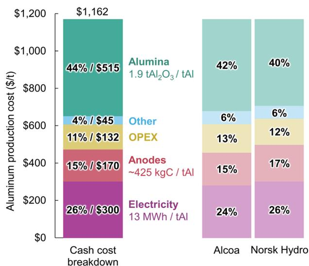
Fig. 3 Aluminum production cost breakdown estimated based on Rio Tinto's total production cost for Canadian smelters,<sup>35</sup> and cost breakdowns from Alcoa<sup>33</sup> and Norsk Hydro.<sup>34</sup> All costs are in US dollars.
