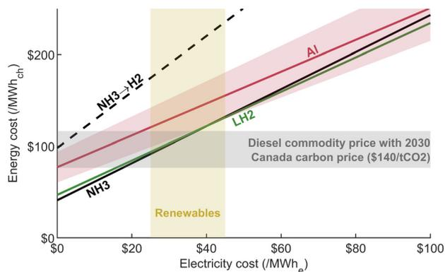
**Fig. 8** PtX cost for all carriers versus electricity cost. The input parameters are set as the average value within their respective range from Table 3. The shaded area for aluminum illustrates the effect of varying the input parameters from the low to high scenario (see Fig. 4), with the number of cycles per year set at 2. Diesel commodity price in the range of \$50–100 per bbl<sup>11</sup> is shown as an indication for the energy cost.
