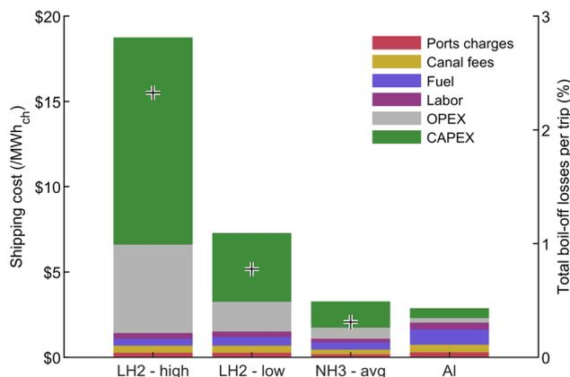
**Fig. 7** Shipping cost breakdown for a 5000 km trip. Both the low and high assumptions of Table 4 are considered for LH<sub>2</sub>, while an average case is used for NH<sub>3</sub>. Crosses show the total boil-off losses per trip, providing insights into the overall transportation efficiency for each pathway.
