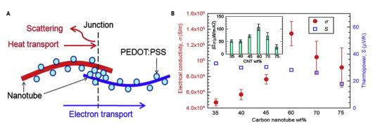
Fig. 8 (A) Graphical representation of the interconnection of CNTs covered by PEDOT:PSS materials. (B) Electrical conductivities and Seebeck coefficients of the composites at various nanotube concentrations, with an inset illustrative of the TE power factor. Adapted with permission from ref. 63. Copyright 2011, American Chemical Society.
