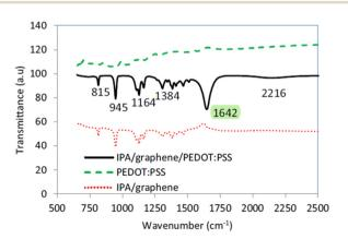
Fig. 9 FTIR spectra of pristine PEDOT:PSS, IPA/graphene/PEDOT:PSS and IPA/graphene solution. 180
