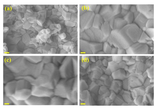
Fig. 3 Scanning electron microscope images of the prepared perovskite thin-films (a) MAPI\_120 °C, (b) MAPI\_MACL\_1, (c) MAPI\_MACL\_2 and (d) MAPI\_MACI\_3 (scale bar is 200 nm for all the images).
