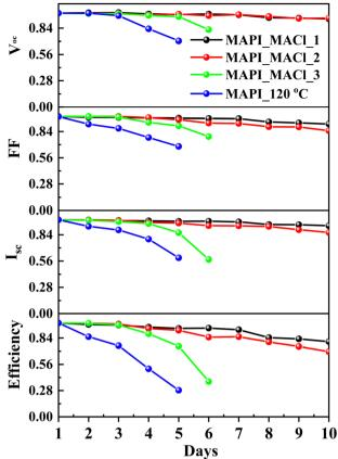
Fig. 7 Stability of the fabricated perovskite solar cells stored under ambient conditions over 10 days (normalized  $V_{\rm oc}$ , FF,  $I_{\rm sc}$  and PCE).
