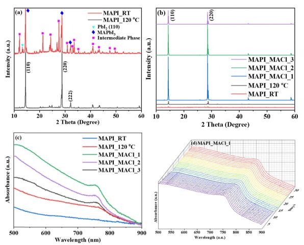
Fig. 2 (a) X-Ray diffraction pattern of MAPI thin-films prepared at room temperature and annealed at 120 °C, (b) XRD patterns of MACI added perovskite thin-films. (c) UV-Vis spectra of prepared perovskite thin-films with different molar amounts of MACI and (d) UV-Vis spectra of MAPI\_MACI\_1 for 32 days stored under ambient conditions at room temperature.
