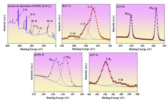
Fig. 4 (a) XPS survey spectrum of MAPI\_MACI\_1 and (b)-(e) high-resolution spectra of C 1s, I 3d, N 1s and Pb 4f, respectively.
