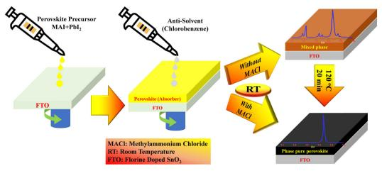
Fig. 1 Schematic representation of room temperature formation of MAPbl<sub>3</sub> perovskite thin-films with the addition of MACl under ambient conditions.
