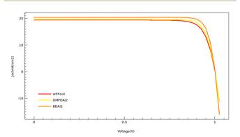
Fig. 5 The J-V curves generated through TCAD simulations are presented for perovskite solar cells (PSCs) without 2D treatment, those treated with BDAI<sub>2</sub>, and those treated with DMPDAI<sub>2</sub>.
