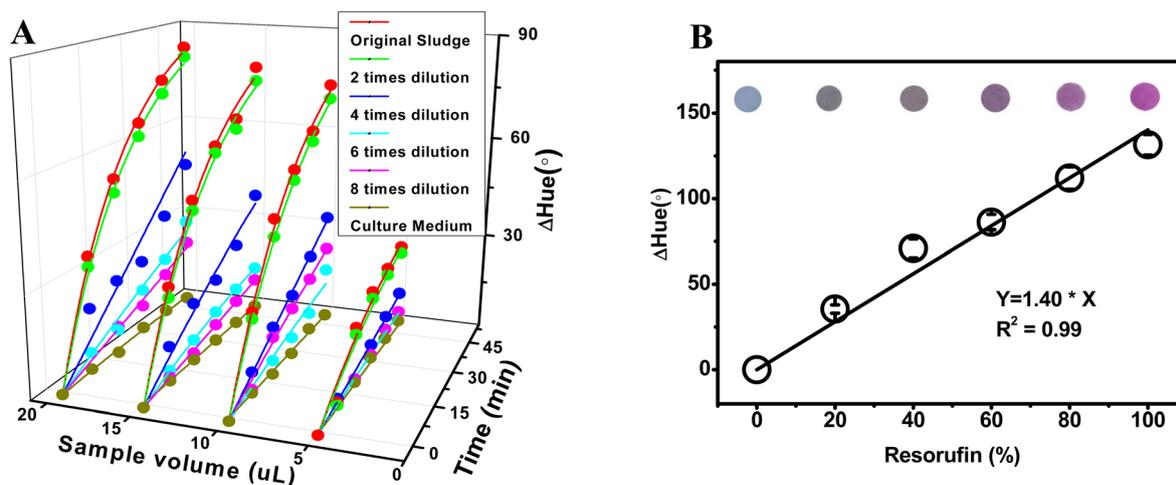
Fig. 3 (A) The effect of sludge sample volume and condensity on speed of color change due to resazurin reduction by anaerobic sludge; (B) the correlation between  $\Delta$ Hue value and resorufin ratio in resorufin/resazurin mixture on Whatman Grade 1 chromatography paper.
