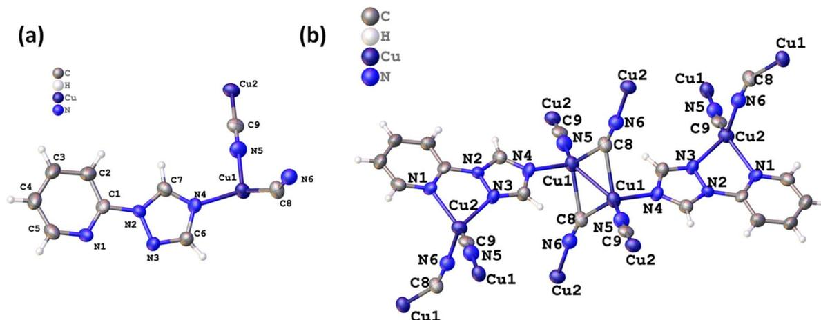
Fig. 1 (a) Asymmetric unit of the 2D MOF, and (b) different coordination modes of CN<sup>-</sup> ions in chain propagation.
