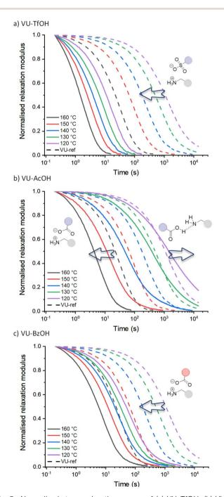
Fig. 3 Normalised stress-relaxation curves of (a) VU-TfOH, (b) VU-AcOH and (c) VU-BzOH measured from 160 to 120 °C and compared to VU-ref (dashed lines). Different viscoelastic behaviour could be observed depending on the acid strength of the additive.
