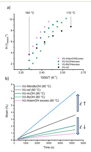
Fig. 6 (a) Arrhenius plot obtained after fitting the relaxation data of the VU materials with an excess of acid additives to a stretched exponential decay. (b) Creep curves at 80 °C, highlighting creep reduction for weaker acids (VU-AcOH, VU-BzOH and VU-AdamOHexcess) and creep increase for more potent acids (VU-NitroBzOH).
