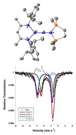
Fig. 5 (Top) ORTEP diagram of  $\bf 8$  with thermal ellipsoids shown at 50% probability and H atoms omitted for clarity; due to apparent disorder in the core, the structure is for connectivity only. (Bottom) Solid state zero-field Mössbauer spectrum of  $\bf 8$  at 80 K. The black circles are the data, the blue and green lines are the components of the fit, the red line is the sum of the components, and the grey line is the residual (data – fit).
