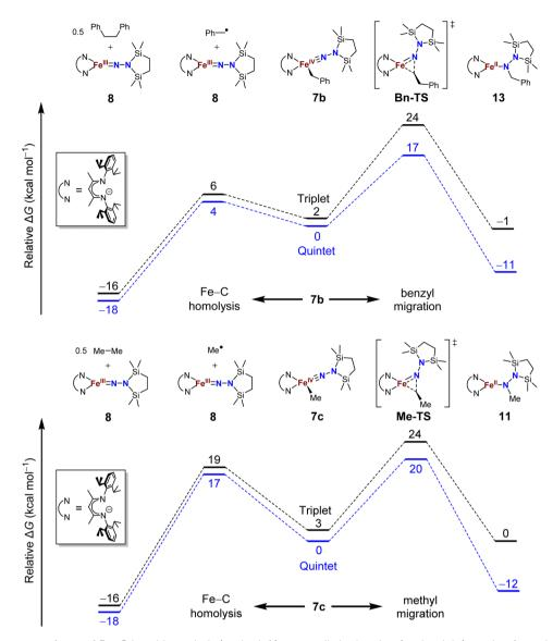
Fig. 9 Potential energy surfaces of Fe-C bond homolysis (to the left) *versus* alkyl migration (to the right) starting from the proposed iron(IV) benzyl (top) and methyl (bottom) complexes from DFT calculations (B3LYP/def2-TZVP).
