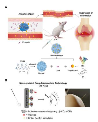
Fig. 7 (A) Therapeutic mechanism of the nano-composite hydrogel (TP@HSA NPs-CCPAGel) against RA. Reproduced from ref. 111 with permission. Copyright 2021, Springer Nature. (B) Schematic of nd-Acu design. Reproduced from ref. 112 with permission. Copyright 2023, Wiley-VCH GmbH.
