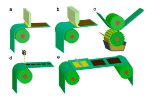
Fig. 19 Common scalable solution processing methods for large-area flexible OSCs which are compatible with roll-to-roll processing. (a) Blade coating, (b) slot die coating, (c) Gravure printing, (d) inkjet printing, (e) screen printing. Reproduced under CC-BY 4.0 License. 165
