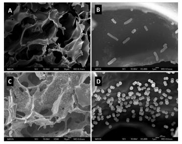
Fig. 16 SEM images of multiple boronic acid ligands containing cryogels with bound E. coli (A) and (B) and S. epidermidis (C) and (D) on. The scale bars are 10 μm in (A) and (C) and 1 μm in (B) and (D). Reproduced under terms of the CC-BY license with permission. 58 Copyright 2022, The Authors, published by the American Chemical Society.
