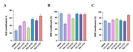
Fig. 34 Drug loading efficiency (DLE) after 24 h of adsorption of HEMA and CD-HEMA cryogels for lomefloxacin (A). Drug release efficiency (DRE) after 24 h in acidic solution (pH = 3, B) and a saline buffer (pH = 7.4, C) of HEMA and CD-HEMA cryogels for lomefloxacin. Reproduced with permission. 96 Copyright 2023, The Royal Society of Chemistry and the Chinese Chemical Society.
