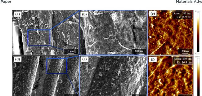
SEM and AFM micrographs of the dominant p- and n-type carbon-based materials, (a)-(c): p-type material, and (d)-(f): n-type material
