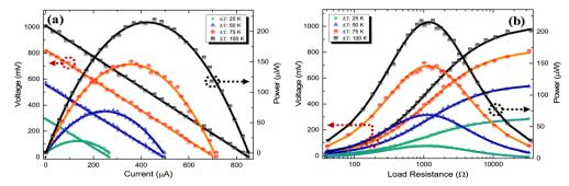
Fig. 6 The thermoelectric performance of the GFRP-GTEG as evaluated experimentally in various  $\Delta T$ s. (a) The obtained curves of voltage-current (V-I), power-current (P-I) and (b) voltage-load resistance ( $V-R_{load}$ ), power-load resistance ( $P-R_{load}$ )
