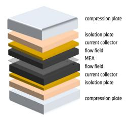
Fig. 9 Visualization of the cell setup.
