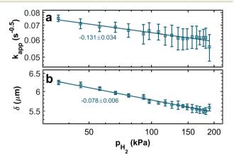
Fig. 8 Double-logarithmic plots of (a) the apparent rate coefficient  $k_{\mathsf{app}}$  and (b) the Nernst diffusion layer thickness  $\delta$  in relation to the hydrogen partial pressure.
