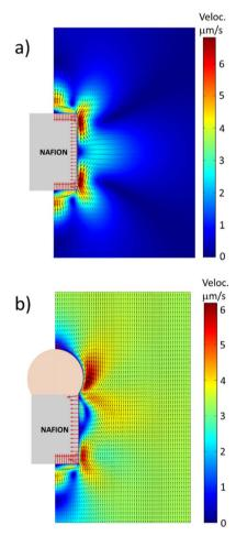
Fig. 3 Numerical simulations for (a) a Nafion rod and (b) a Nafion rod capped by a passive sphere. The figure shows the electric field (red arrows) and the stationary velocity field (black arrows), plotted in the reference system of the Nafion. The colour scale represents the magnitude of the velocity.
