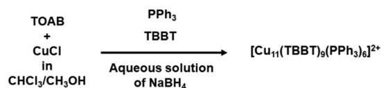
Fig. 6 Synthesis procedure of [\text{Cu}_{11}(\text{TBBT})_9(\text{PPh}_3)_6]^{2+} NC.
