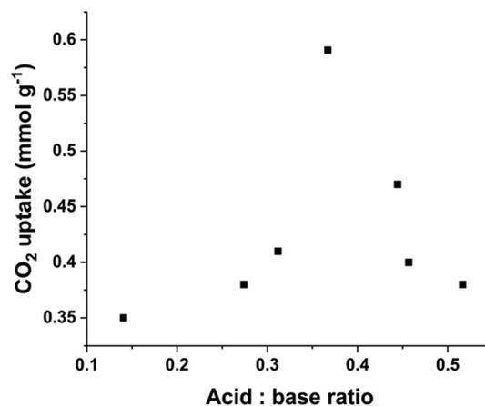
Fig. 5 CO<sub>2</sub> capture as a function of acid : base ratio of LDOs calcined at 400 °C.
