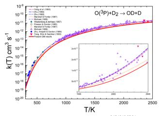
Fig. 10 Comparison of individual measurements<sup>8,13,15,19,23,24</sup> and global fits  $^{15,16,19,23}$  of rate coefficients for the O + D $_2$  reaction. The inset shows a blow-up of the 1500-2500 K range. The red solid line represents the present QM k(T).
