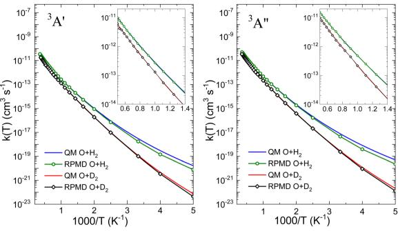
Fig. 6 QM and RPMD rate coefficients for  $O(^3P) + H_2$  and  $O(^3P) + D_2$  reactions on  $^3A''$  (left) and  $^3A''$  (right) PESs. No electronic partition function is included. Note the excellent agreement between the QM and RPMD for the  $O(^3P) + D_2$  reaction on both PESs.
