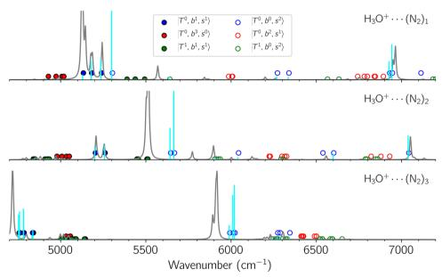
Fig. 5 Calculated spectra from the FBR Hamiltonian with (grey line) and without off-diagonal coupling (cyan sticks) for  $H_3O^+\cdots(N_2)_n$ . The filled and empty circles represent the diagonal energies of bright states  $|T^0, b^1, s^1\rangle$  and  $|T^0, b^0, s^2\rangle$ , and the relevant states lighted up by them, respectively, which show the locations of these states without mechanical anharmonicity.
