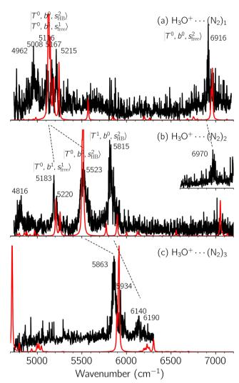
Fig. 2 Observed (black) and calculated (red) NIR spectra of  $H_3O^+\cdots(N_2)_n$ . (a) n=1, (b) n=2, and (c) n=3, in the OH stretching overtone region. The  $N_2$ -loss fragmentation channel was monitored to record the observed spectra (a) and (b). Observed spectrum (c) and the inset spectrum (b) were obtained by monitoring the  $2N_2$ -loss fragmentation channel.
