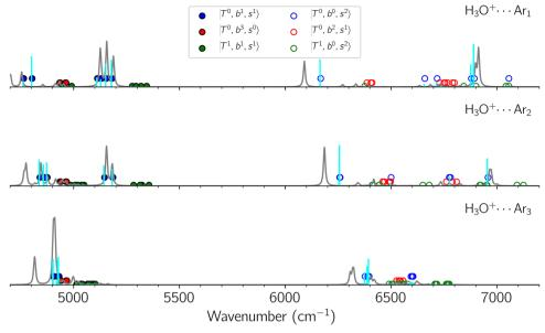
Fig. 4 Calculated spectra from FBR Hamiltonian with (grey line) and without off-diagonal coupling (cyan sticks) for H<sub>3</sub>O<sup>+</sup>···Ar<sub>n</sub>. The filled and empty circles represent the diagonal energies of bright states  $|T^0, b^1, s^1\rangle$  and  $|T^0, b^0, s^2\rangle$ , and the relevant states lighted up by them, respectively, which show the locations of these states without mechanical anharmonicity.
