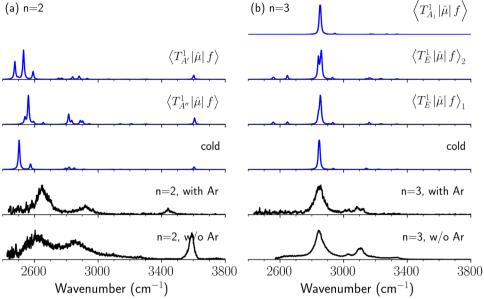
Fig. 7 Comparison among the observed cold (Ar-tagged) and warm (bare) spectra and calculated cold and hot band spectra of  $H_3O^+\cdots(CO)_n$ , (a) n=2 and (b) n=3, in the OH stretch fundamental region. In the hot band spectrum simulation, transitions from the first excited level of the OH...CO hydrogen-bond stretching modes ( $T_{A'}$  and  $T_{A''}$  for n=2,  $T_{A_3}$  and degenerated  $T_E$  for n=3) are calculated.
