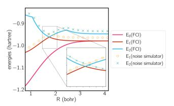
Fig. 2 Potential energy curve calculated by FCI and the noise simulator. Molecule is treated in the  $C_{2v}$  symmetry, where the polar coordinates of the three hydrogen atoms are (1,0), (1, $\pi$ ) and (R, $\pi$ /2).
