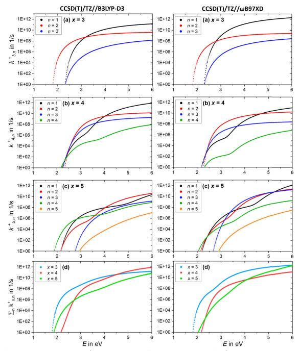
Fig. 8 (a)–(c) Calculated RRKM rate constants  $k_{X,n}^+$  for the loss channels (2) of the precursor ions (NaCl)<sub>x</sub>Na<sup>+</sup> with x = 3-5. Note that the loss channels producing  $Na^+$  ions  $(k_{x,n=x}^+)$ , which cannot be detected in the experiment, are always the slowest at higher energies. (d) Total fragmentation rate constants  $\sum k_{x,n}^+$  as sum of all loss channels *n* for cluster sizes x = 3-5.
