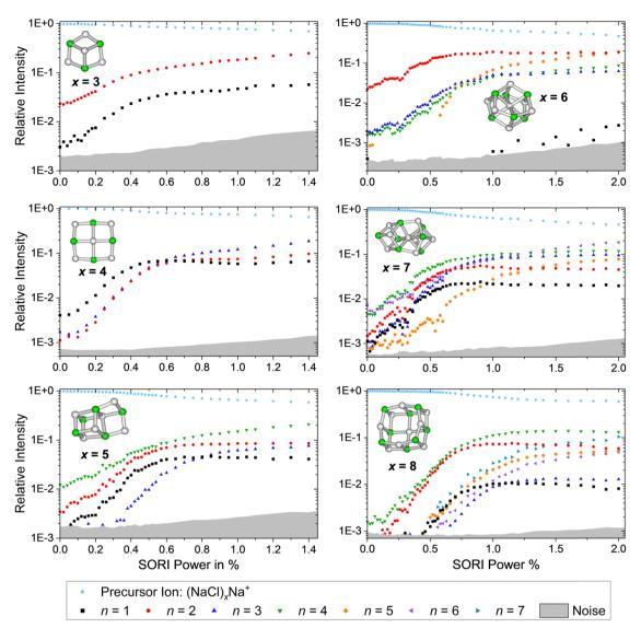
SORI CID spectra of the sodium chloride cluster ions  $(NaCl)_xNa^+$  with x = 3-8. The stoichiometric loss channels (2) are observed
