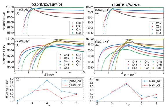
Fig. 7 Relative density of states (DOS) of the cationic clusters (NaCl)<sub>x</sub>Na<sup>+</sup> with (a) x = 3 and (b) x = 4. The isomers considered are shown in Fig. 1 and Fig. S1 (ESI†). (c) The energy needed to redistribute 25% of the lowest energy isomer into higher-lying isomers as a function of the cluster size x for anions and cations
