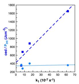
Fig. 8 Properties ced (J cm $^{-3}$ ) dark blue squares and  $P_{int}$  (J cm $^{-3}$ ) light blue circles relative to  $k_1$  (10<sup>-7</sup> s<sup>-1</sup>)<sup>25</sup> in benzene, ethanol, acetonitrile and  $[C_4C_1im][NTf_2]$  for reaction  ${f B}$
