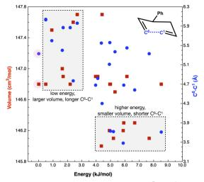
Fig. 7 Reaction **B** reactant conformer volume (cm<sup>3</sup> mol<sup>-1</sup>) red squares and C<sup>1</sup>-C<sup>6</sup> distance (Å) blue circles vs. relative energy (kJ mol<sup>-1</sup>). Pink shaded circles indicate the lowest energy conformer. Grey boxes highlight two different domains.
