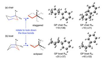
Fig. 4 Reaction B (a) chair and (b) boat TS conformers, chem draw and optimised GP structures, Gibbs free energy  $\Delta G_{act}$  for the chair-equatorial conformer and relative  $\Delta G$  to the chair-equatorial conformer for the other TSs at the B3LYP (M06-2X) level in kJ  $mol^{-1}$ .
