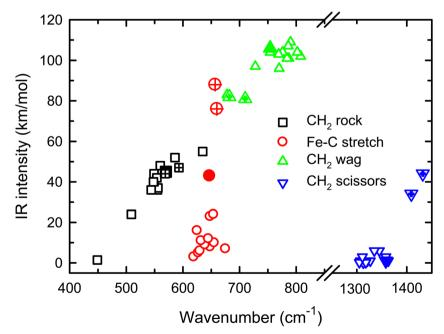
Fig. 3 Theoretical IR intensities versus wavenumber for the four vibrations accessible experimentally in the present experiments. CCSD results are closed symbols and MP2 results are hatched
