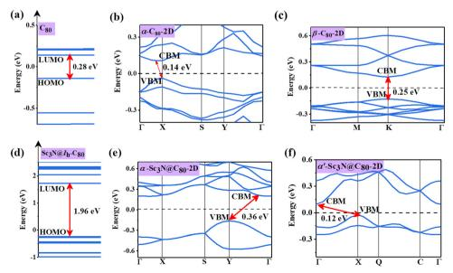
Fig. 4 Electronic structures of (a)  $C_{80}$  fullerene, (b)  $\alpha$ - $C_{80}$ -2D, (c)  $\beta$ - $C_{80}$ -2D, (d)  $Sc_3N@I_n$ - $C_{80}$  fullerene, (e)  $\alpha$ - $Sc_3N@C_{80}$ -2D, and (f)  $\alpha'$ - $Sc_3N@C_{80}$ -2D. The Fermi level is set to zero
