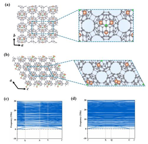
Fig. 2 Crystal structures and phonon dispersions of monolayers (a) and (c)  $\alpha$ -Sc<sub>3</sub>N@C<sub>80</sub>-2D and (b) and (d)  $\alpha'$ -Sc<sub>3</sub>N@C<sub>80</sub>-2D, where grey, orange and green denote C, Sc and N atoms.
