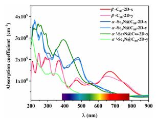
Fig. 5 Optical absorption coefficients of  $\beta$ -C<sub>80</sub>-2D,  $\alpha$ -Sc<sub>3</sub>N@C<sub>80</sub>-2D and  $\alpha'$ -Sc<sub>3</sub>N@C<sub>80</sub>-2D monolayers calculated by the HSE06 functional. The wavelength range of the visible light region (380-780 nm) is in iridescent color.
