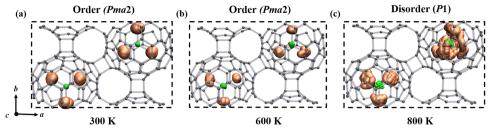
Fig. 3 Schematic representation of order–disorder states of the  $\alpha$ -Sc<sub>3</sub>N( $\alpha$ C<sub>80</sub>-2D crystal driven by temperature at (a) 300 K, (b) 600 K, and (c) 800 K. The representative rotational operation of the  $Sc_3N$  species for the  $\alpha$ - $Sc_3N$ ( $\alpha$ C $_{80}$ -2D phase is available in the movies of the ESI.†
