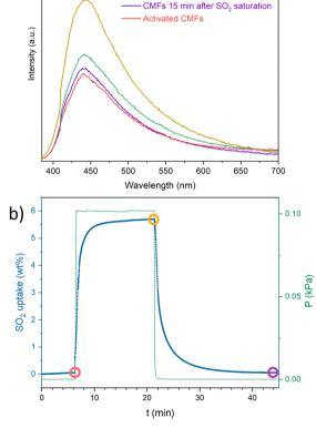
Fig. 4 (a) Photoluminescence CMFs spectra ( $\lambda_{ex}$  = 370 nm) of as synthesised, activated, SO<sub>2</sub> saturated and after the exposure to SO<sub>2</sub> samples. (b) Profile of adsorption–desorption kinetics of SO<sub>2</sub> on CMFs (gravimetric experiment with controlled SO<sub>2</sub> atmosphere).
