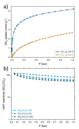
Fig. 3 (a) Comparison of the  $SO_2$  and  $CO_2$  adsorption isotherms at 298 K on CMFs. (b) IAST selectivity of  $SO_2/CO_2$  on MCFs for different concentrations of the binary mixture.
