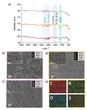
Fig. 2 (a) IR-ATR spectra at different stages according to the points marked in Fig. 1b, pristine sample (pink), after SO<sub>2</sub> uptake (yellow), and after 10 desorption cycles (violet). SEM micrographs with their EDX results on (b) pristine sample, (c) after 10 desorption cycles, (d) after SO<sub>2</sub> uptake, and (e) the EDX mapping results of the rectangular area inside panel (d).
