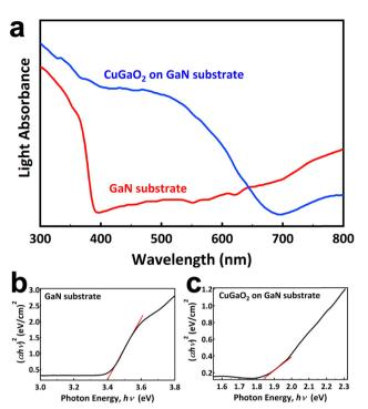
Fig. 4 (a) UV-Vis diffused reflectance spectra of the GaN substrate and CuGa<sub>2</sub>O<sub>4</sub> on GaN, and bandgap estimation of (b) the GaN substrate and (c) CuGaO2 on GaN samples.
