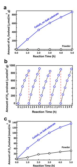
Fig. 5 (a) Photocatalytic hydrogen generation of powder and CuGaO<sub>2</sub> on GaN samples, (b) three cycles for the stability test of hydrogen generation of the CuGa<sub>2</sub>O<sub>4</sub> on GaN sample, and (c) photocatalytic oxygen generation of powder and CuGaO2 on GaN samples.
