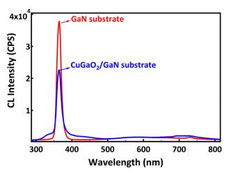
Fig. 6 Cathodoluminescence spectra acquired for each sample.
