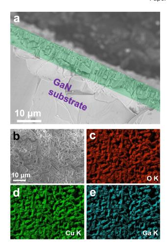
Fig. 3 (a) SEM cross-section image of the film on the substrate, (b) SEM micrograph of the film surface, and EDS mapping of the corresponding elements (c) O K $\alpha$ , (d) Cu K $\alpha$ , and (e) O K $\alpha$ .
