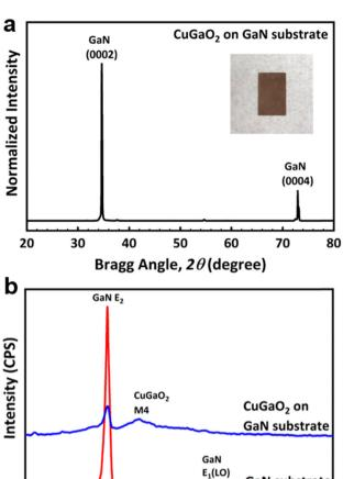
Fig. 2 (a) XRD profile of a CuGaO<sub>2</sub> film grown on the GaN substrate with a digital photograph of it in the inset, and (b) Raman spectra of the GaN substrate before and after epitaxial growth.
