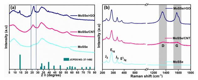
Fig. 4 (a) PXRD pattern and (b) Raman spectra of the bare MoSSe, MoSSe@CNT and MoSSe@RGO heterostructure.
