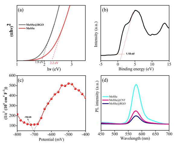
Fig. 7 (a) Tauc plot of MoSSe and the MoSSe@RGO nanocomposite; (b) VB XPS spectra and (c) Mott-Schottky plots of the MoSSe@RGO nanocomposite; (d) PL spectra of an aqueous solution of eosin Y  $(1.0 \times 10^{-7} \text{ M}, \text{ excitation wavelength} = 490 \text{ nm})$  in the presence of MoSSe@CNT and MoSSe@RGO
