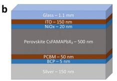
Fig. 2 (a) ANU perovskite solar cell structure. (b) Caelux perovskite solar cell structure
