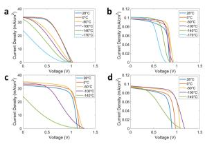
Fig. 3 Pre-radiation LILT J-V curves for (a) ANU9 cell at 1.0 AU, (b) ANU9 cell at 19.2 AU, (c) Caelux CA3 cell at 1.0 AU, and (d) Caelux CA3 cell at 19.2 AU.
