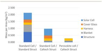
Fig. 1 Comparison of the mass per area of current state-of-the-art solar cells with perovskite solar cells. The perovskite solar cell structure assumes no coverglass (due to the radiation hardness of perovskites) and a value of 0.0056 kg m<sup>-2</sup> for the PSC, which is too small of a contribution to be visible in the figure.
