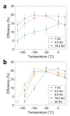
Fig. 4 Plots of average efficiency with respect to temperature at various light intensities for (a) ANU perovskite solar cells and (b) Caelux perovskite solar cells, both before radiation. The error bars denote the standard deviation in the set of measurements (n = 3 cells in each case).
