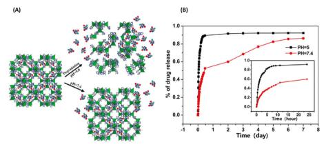
Fig. 6 ZIF-8 as a pH-sensitive delivery vehicle for the controlled release of 5-fluorouracil (5-FU). (A) The scheme of pH-response of the encapsulated 5-Fu release from ZIF-8; (B) the NIM release process in physiological saline at 37 °C. 32 Copyright 2014, Dalton Transactions.
