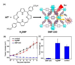
Fig. 18 MOFs constructing with porphyrin derivative-based linkers for highly efficient PDT. (A) Synthesis of Hf-DBP NMOF and the schematic description of the <sup>1</sup>O<sub>2</sub> generation process. (B) Tumor growth inhibition curve after PDT treatment. Black and red arrows refer to injection and irradiation time points, respectively. (C) Tumor weight after PDT treatment. 143 Copyright 2014, Journal of the American Chemical Society.
