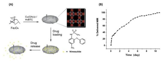
Fig. 4 Fe<sub>3</sub>O<sub>4</sub>@MOF for magnetic targeted drug delivery and controlled release. (A) The synthesis and action of Fe<sub>3</sub>O<sub>4</sub>/Cu<sub>3</sub>(BTC)<sub>2</sub> nanocomposites for potential targeted drug release; (B) the NIM release process in physiological saline at 37 °C. 29 Copyright 2011, Journal of Materials Chemistry.
