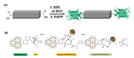
Fig. 11 The bioconjugation of proteins onto the surface of MOFs via functional groups of the organic linkers. (A) The bioconjugation of the 1D-MOFs,  $[(Et_2NH_2)(In(pda)_2)]_n$  with EGFP. <sup>89</sup> Copyright 2011, Chemical Communications (Camb). (B) Trypsin immobilization onto DCC-activated MIL-88B-NH2. <sup>90</sup> Copyright 2012, ChemPlusChem.
