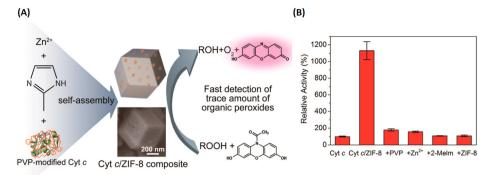
Fig. 10 ZIF-8 for enzymes and functional proteins delivery. (A) Preparation of the Cyt c-embedded ZIF-8 and its biocatalysis. (B) The relative peroxidase activity of Cyt c, Cyt c/ZIF-8 composite, PVP/Cyt c mixture, Cyt c/zinc ion mixture, Cyt c/2-methylimidazole mixture, and Cyt c/ZIF-8 mixture. Telephone activity of Cyt c, Cyt c/ZIF-8 composite, PVP/Cyt c mixture, Cyt c/zinc ion mixture, Cyt c/2-methylimidazole mixture, and Cyt c/ZIF-8 mixture. Copyright 2014, Nano Letters.
