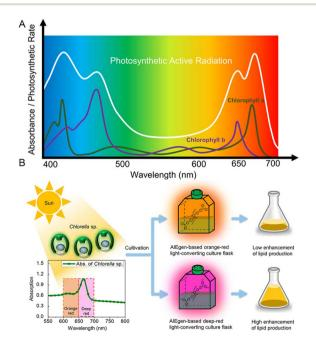
**Fig. 7** (A) The absorption spectra of chlorophyll and photosynthetically active radiation (PAR). (B) Schematic illustration showing that *Chlorella* sp. can utilize the solar energy more efficiently in the AIEgenbased deep-red light-converting culture flask. Reproduced with permission from ref. 71. Copyright 2020, American Chemical Society.
