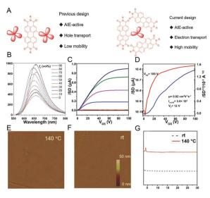
Fig. 16 (A) The design principles of AlEgen-based OFET devices. (B) TriPE-3PDI in CHCl<sub>3</sub>/hexane mixtures with different hexane fractions ( $f_h$ ). (C) Transfer and (D) output characteristics for OTFT devices of TriPE-3PDIL annealed at 140 °C. AFM images of TriPE-3PD at (E) 140 °C and (F) at room temperature. (G) XRD patterns of thin films of TriPE-3PDIL at room temperature and 140 °C. Reproduced with permission from ref. 176. Copyright 2018, Wiley-VCH.
