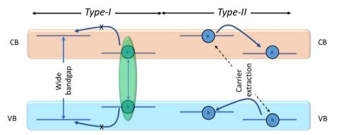
Scheme 1 A schematic representation of type-I and type-II heterojunctions in typical core/shell nanostructures.
