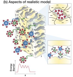
(a) Illustration of the treatment of ion transport by the Donnan steric pore model with dielectric exclusion (top) and solution-diffusion model (bottom) compared to (b) a more realistic model of ion transport with more accurately determined parameters for ion size, void size distribution, and dielectric constant that accounts for interactions and resistances that an ion experiences at the surface and interior regions of the membrane
