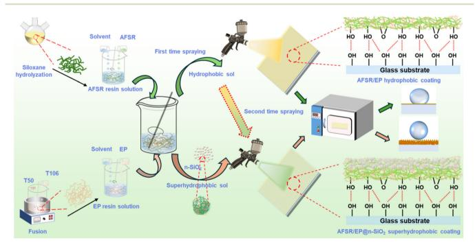
Scheme 1 The fabrication process of AFSR/EP hydrophobic coating and AFSR/EP@n-SiO₂ superhydrophobic coating
