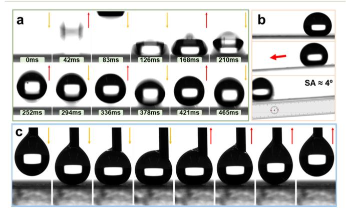
Fig. 7 Analysis of dynamic behaviour of water droplets. (a) Images demonstrate the repeating bounce behavior of a 15 µL water droplet on a horizontally placed spray-coated glass. (b) The SA test result of AFSR/EP@n-SiO<sub>2</sub> coatings with a 15 µL water droplet. (c) The test process of non-stacking property of AFSR/EP@n-SiO<sub>2</sub> coatings towards the water droplet using a contact angle measuring instrument.
