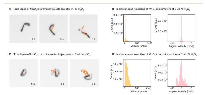
Fig. 5 Motion characterization of MnO<sub>2</sub> and MnO<sub>2</sub>/Lac micromotors at 2 wt% H<sub>2</sub>O<sub>2</sub>. (A) Time-lapse of MnO<sub>2</sub> micromotors trajectories. (B) Velocities and angular velocities for MnO<sub>2</sub> micromotors. (C) Time-lapse of MnO<sub>2</sub>/Lac micromotors trajectories. (D) Velocities and angular velocities for MnO<sub>2</sub>/
