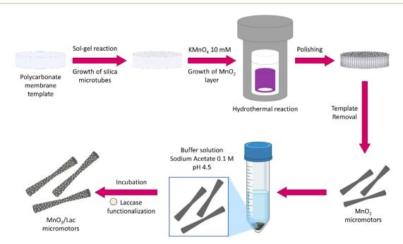
Fig. 2 Fabrication of MnO<sub>2</sub>-based micromotors by wet chemical methods followed by laccase immobilization.
