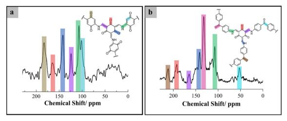
Fig. 2 Structural characterization of the COF structure: (a) <sup>13</sup>C CP-MAS solid-state NMR spectra of HqTpCOF and (b) <sup>13</sup>C CP-MAS solid-state NMR spectra of BpTpCOF.
