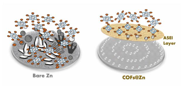
Fig. 8 Scheme illustrates the function of COFs as an ASEI for the Zn anode.
