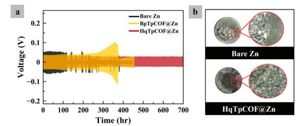
Fig. 4 (a) Long-term GCD profiles of the bare Zn electrode and COF layer coated on the Zn electrode at a current density of 1 mA cm<sup>-2</sup> and a capacity of 1 mA h cm<sup>-2</sup> and (b) surfaces of different electrodes after battery failure.
