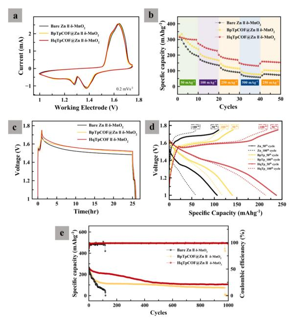
Fig. 9 Electrochemical performances of bare Zn// $\delta$ -MnO<sub>2</sub>, BpTpCOF@Zn// $\delta$ -MnO<sub>2</sub>, and HqTpCOF@Zn// $\delta$ -MnO<sub>2</sub> full cells: (a) CV profiles at 0.2 mV s<sup>-1</sup>, (b) rate capability at various current densities, (c) self-discharge performance of full cells, (d) charge-discharge profiles at 50 and 100 cycles, and (e) cycling stability at a current density of 250 mA g<sup>-1</sup>.
