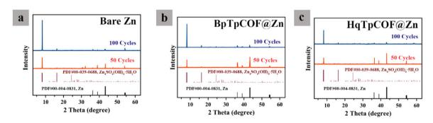
Fig. 6 XRD patterns of different anodes: (a) bare Zn, (b) BpTpCOF@Zn, and (c) HqTpCOF@Zn
