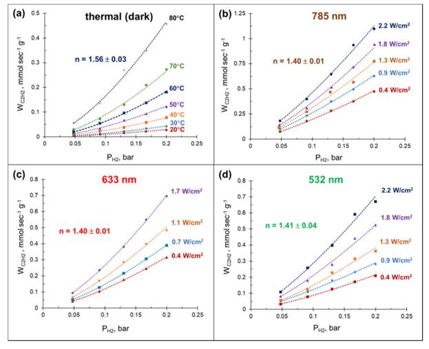
Fig. 4 Acetylene conversion rate over 3%Pd-Mg/GS as a function of hydrogen partial pressure  $P_{\rm H_2}$ . (a) Thermal (dark) and photo mediated with laser light illumination wavelengths of (b) 785 nm, (c) 633 nm, and (d) 532 nm. The  $P_{\rm C_2H_2}$  was kept constant at 0.05 bar and the reaction order (n) reported is with respect to H<sub>2</sub>.
