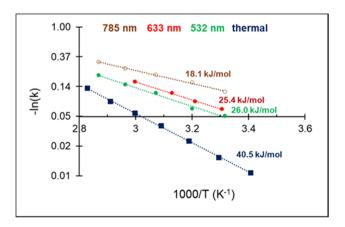
Fig. 5 Arrhenius plot of C<sub>2</sub>H<sub>2</sub> hydrogenation and apparent activation energies for photo- and thermocatalytic experiments over 3%Pd-Mg/
