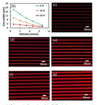
Fig. 1 (a) Schematic illustration of the EHD printing system comprising a single nozzle, a movable platform, a conductive platform and a power supply system, (b) and (c–g) fluorescence images of patterned lines with QD ink of 6 cP at printing speeds of 10 mm s<sup>-1</sup>, 7 mm s<sup>-1</sup>, 5 mm s<sup>-1</sup>, 3 mm s<sup>-1</sup> and 1 mm s<sup>-1</sup>, respectively.
