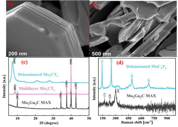
Fig. 7 SEM images of the (a) Mo<sub>2</sub>Ga<sub>2</sub>C Max phase, (b) after HF etched Mo<sub>2</sub>CT<sub>x</sub> MXene, (c) XRD pattern of Mo<sub>2</sub>Ga<sub>2</sub>C during HF etching, (d) Mo<sub>2</sub>Ga<sub>2</sub>C MAX phase and delaminated Mo<sub>2</sub>CT<sub>x</sub> MXene Raman spectra. Reprinted with permission from ref. 130. Copyright 2020 American Chemical Society
