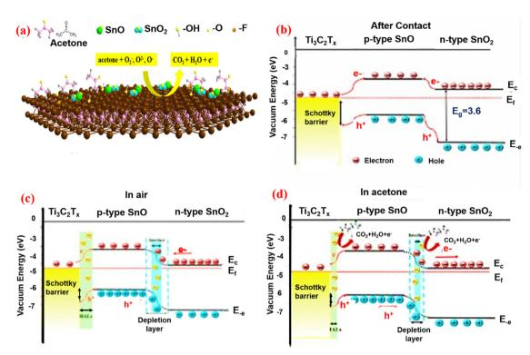
Fig. 8 Schematic illustration of the band diagram of the p-n heterojunction and the combination of the SnO-SnO<sub>2</sub>/Ti<sub>3</sub>C<sub>2</sub>T<sub>y</sub> sensor. Adopted with permission from ref. 139. Copyright 2020 Material Science Technology.
