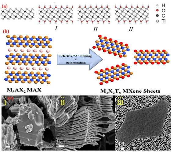
Fig. 4 (a) Configuration of the OH groups: (i)  $Ti_3C_2(OH)_2$ , (ii)  $Ti_3C_2(OH)_2$ . Adopted with permission from ref. 73. Copyright 2012, Computational and Theoretical Chemistry, Elsevier. (b) Schematic illustration of the MXene synthesis process from the MAX phase. (ii) MAX phase, (iii) Multilayer MXene, and (iii) MXene assembled flakes in a colloidal solution. Adopted with permission from ref. 62. Copyright 2017, American Chemical Society.
