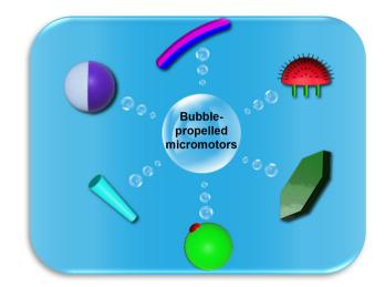
Fig. 1 Schematic of the morphology of various micromotors designed for bubble propulsion: clockwise from the top, Janus rod, 64 jellyfish, 55 hexagon, <sup>58</sup> eccentric Janus, <sup>54</sup> tube, <sup>45,65,66</sup> and Janus sphere. <sup>40,56,59,67–69</sup>
