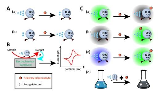
Fig. 2 Sensing mechanism. (A) Motion-based-sensing. (a and b) Decrease and increase in speed of motors upon sensing the targets. (B) Micromotorassisted electrochemical detection. (C) Optical detection of analytes: fluorescence-based detection and colorimetric assay. (a) Fluorescence quenching (b) Fluorescence recovery. (c) Ratiometric fluorescence response. (d) Naked-eye colorimetric assay.
