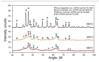
Fig. 1 XRD patterns of Ni/Fe oxide materials after calcination at 350 °C, 450 °C and 500 °C.
