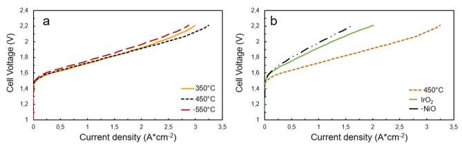
Fig. 6 Comparison of I-V curves at 60 °C (a) among the differently treated NiFeOx-based cells and (b) among the cells equipped with NiFe-oxide 450, IrO2, and NiO at the anode.
