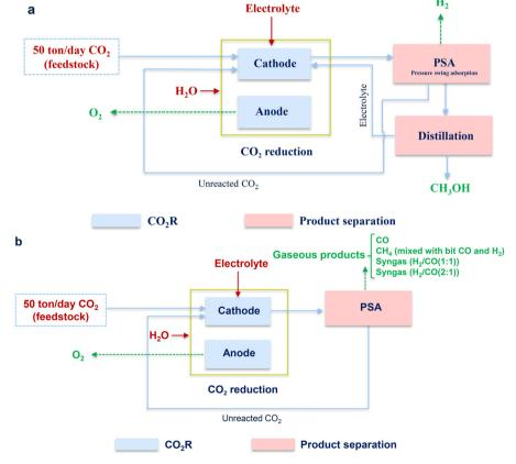
Fig. 4 The flow diagram of CO<sub>2</sub>R to CH<sub>3</sub>OH (a) and gaseous products (b).
