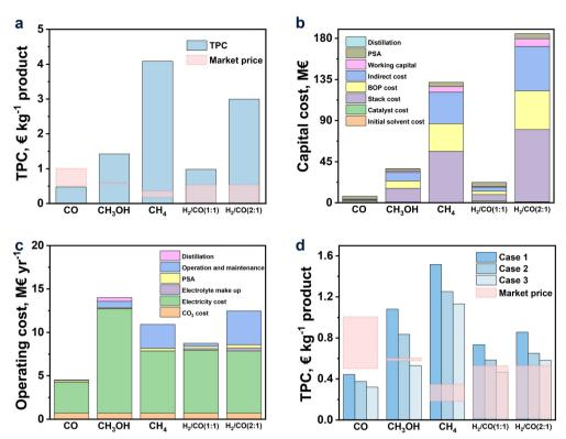
Fig. 5 (a) TPC; (b) capital cost and (c) operating cost for  $CO_2R$  to CO,  $CH_3OH$ ,  $CH_4$ , and syngas  $(H_2/CO \ (1:1) \ and \ H_2/CO \ (2:1))$  in the base case; (d) TPC for each product in the future cases.
