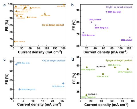
Fig. 1 Performance, including FE and current density, of CO<sub>2</sub>R to CO (a); CH<sub>3</sub>OH (b); CH<sub>4</sub> (c); and syngas (d) in the IL-base electrolytes.
