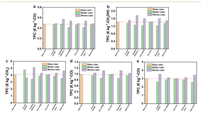
Fig. 6 Sensitivity analysis for CO<sub>2</sub>R to C1 products under better and worse cases with different parameters, (a) CO; (b) CH<sub>3</sub>OH; (c) CH<sub>4</sub>; (d) syngas of H2/CO (1:1) and (e) syngas of H2/CO (2:1).
