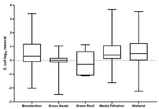
Fig. 1 Log removal of *E. coli* through GSI systems, including bioretention (n = 122), grass swales (n = 39), green roofs (n = 6), media filtration (n = 104), and wetlands (n = 270). Data was accessed from the International Stormwater BMP database on May 1, 2023.
