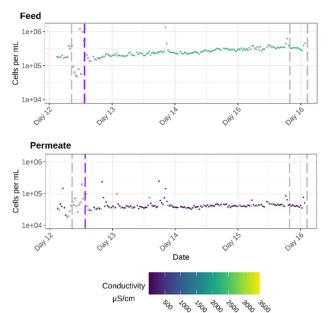
Fig. 4 Overview of the cell densities (cells per mL) and conductivity values (colour-scale) in the feed (top) and permeate (bottom) stream right before and during the days after the ultrasound treatment (purple dashed line). The grey lines mark flushes. If the pilot is not in operation conductivity was not measured and therefor given in grey (hollow points).
