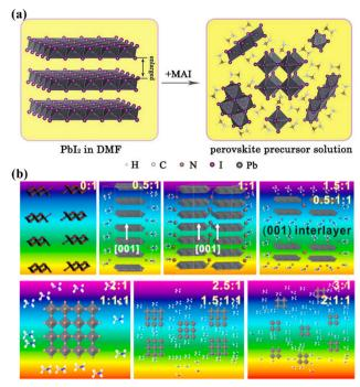
Fig. 3 (a) Schematic of the evolution of lead-iodine complexes after MAI addition.<sup>53</sup> Copyright 2019, Wiley-VCH Verlag. (b) Types of lead iodine complexes that may occur in precursors with different MAI/PbI2 mole ratios. 55 Copyright 2015, American Chemical Society.
